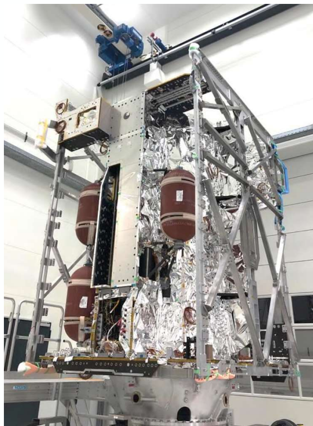
FM primary structure at ArianeGroup Lampoldshausen for Chemical Propulsion System (CPS) integration
